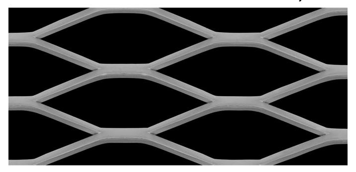
LW Pitch:121.92mmStrand Width:6.35mmSW Pitch:33.84mmThickness:5.00mmWeight:5.06 kg / m2Open Area:63%
